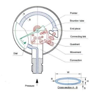
The Bourdon tube pressure gauge operates on the principle, the when the gauge is pressurized, a flattened tube tends to straighten or regain its circular form. Most Bourdon tube gauges employ the C shape, which is the type of Bourdon pictured above.
