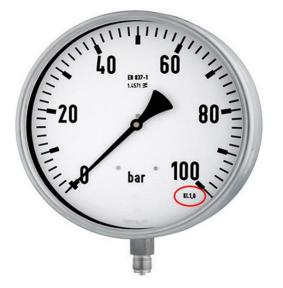
The accuracy class is shown on the dial as Acc, Class, Cl or Kl (e.g. Cl 1.0 for 1% of full scale value).
